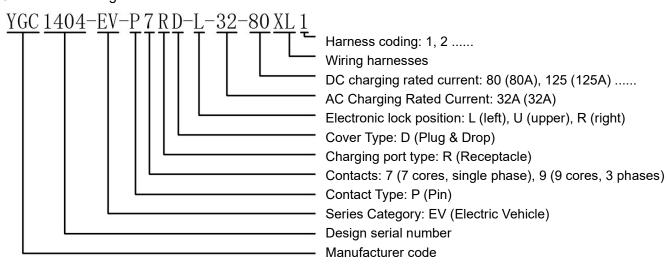
For example: YGC1404-EV-P7RD-L-32-80 means, YG1404 European standard DC 80A AC 32A single-phase, electronic lock arrangement on the left side of the integrated charging receptacle.
