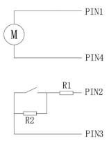
★ Note: Conventional switching feedback without resistance scheme can be selected according to customer needs.
