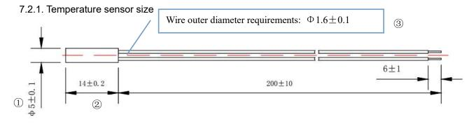
★ Note: (1), (2) and (3) are required sizes, and the rest of the sizes can be customized
